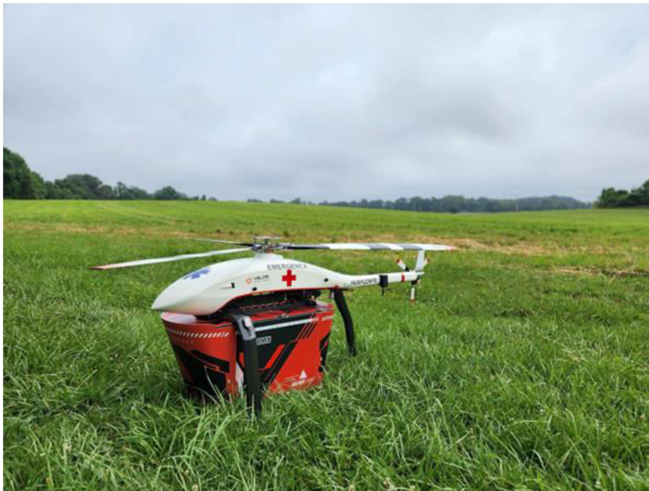
Figure 1: Velos helicopter-style drone used in a 100-mile organ drone run in southern Maryland. The craft is all electric, supports \approx 20 kg and can reach speeds of 50–70 mph depending on ambient conditions and payload weight. With kind permission from Dr Joseph Scalea, Professor of Transplant Surgery, Charleston, SC, USA [20].
